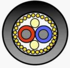
Part Number: 46349CH.001000 MCROPHONE CABLE 24AWG FRNC/LSZH-C
